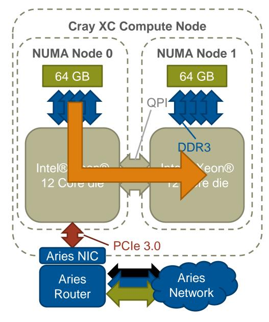
The design of the XC node means that CPUs accessing data stored on the other socket/die have to cross the QPI interprocessor bus
