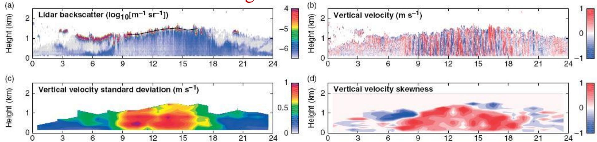
Skewness of vertical velocity distribution from doppler lidar distinguishes surface-driven vs. cloud-top driven turbulence
