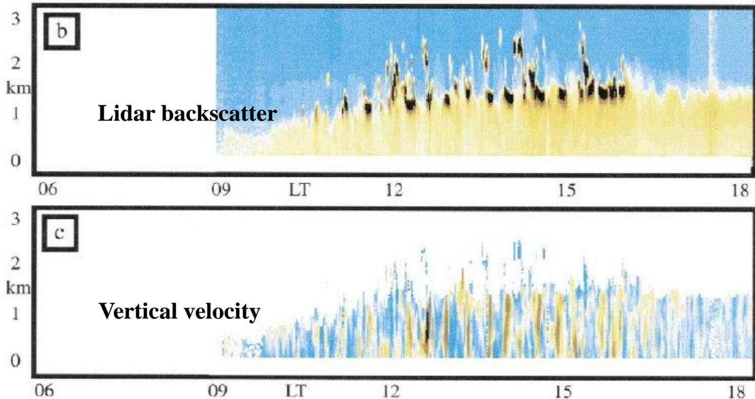
In addition to backscatter, get vertical velocity from doppler lidar. Helps define BLH, but also provides information on **turbulent motion**
