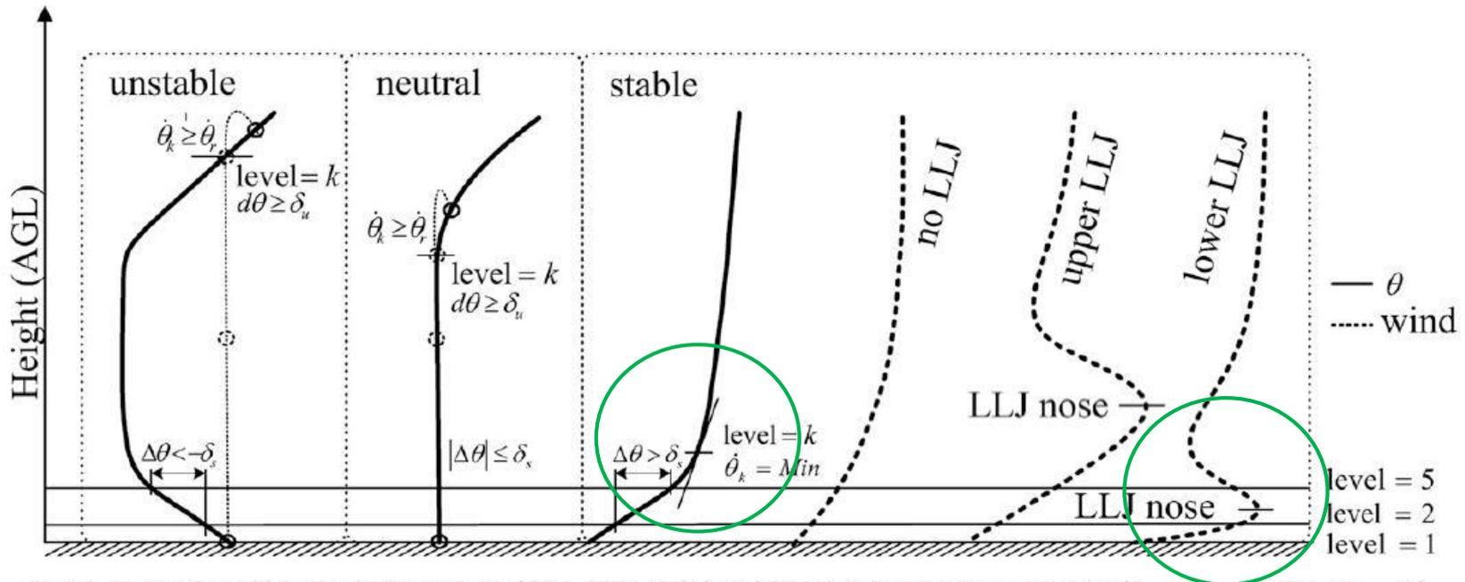
FIG. 3. Illustration of idealized PBL regimes (CBL, NRL, SBL) and PBLH determination procedure ( $\Delta\theta = \theta_5 - \theta_2$ ;  $d\theta = \theta_k - \theta_1$ ).
