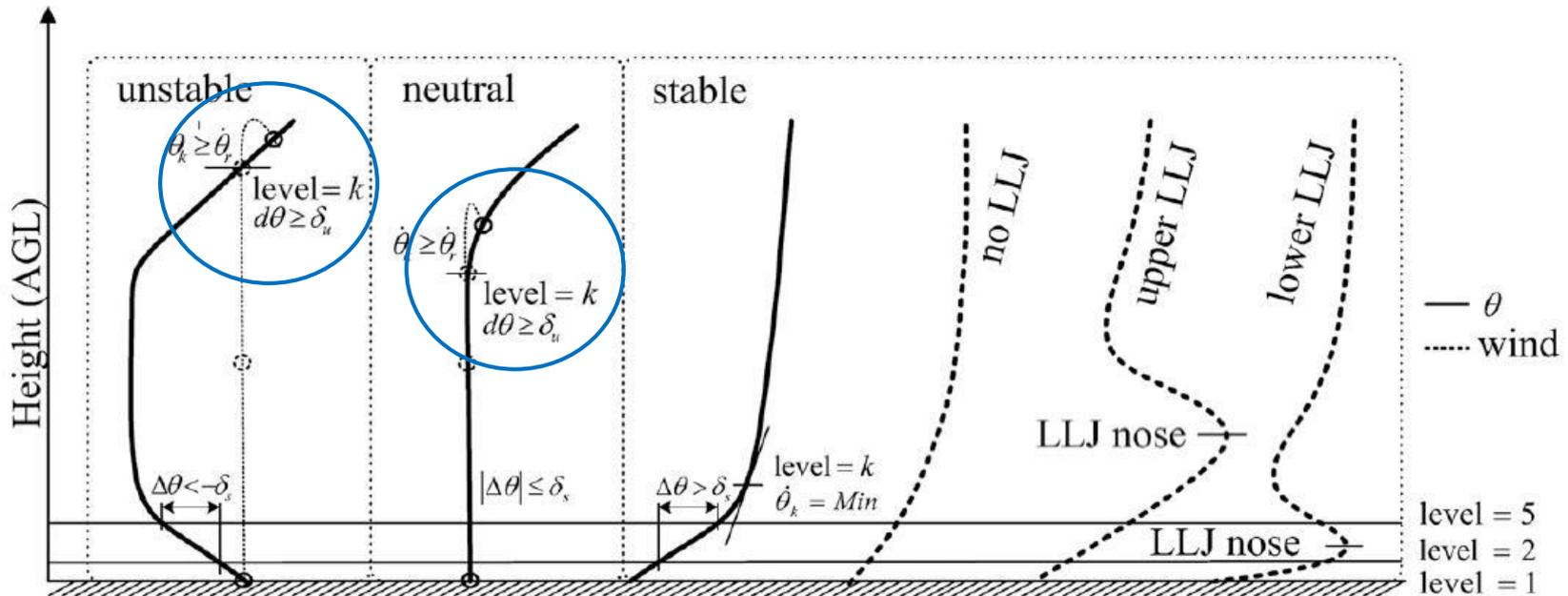
FIG. 3. Illustration of idealized PBL regimes (CBL, NRL, SBL) and PBLH determination procedure ( $\Delta\theta = \theta_5 - \theta_2$ ;  $d\theta = \theta_k - \theta_1$ ).
