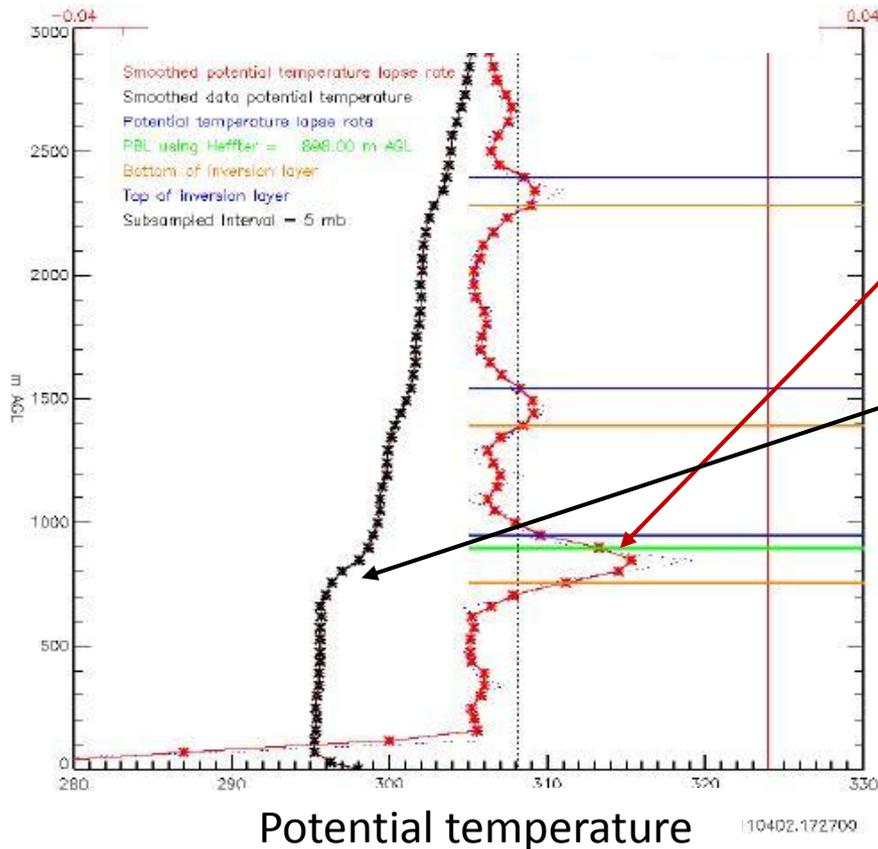
*Figure 1: PBL determination using Heffter method when the profile was subsampled and smoothed at 5 mb and 15 mb respectively at SGP on April 02, 2011.*
