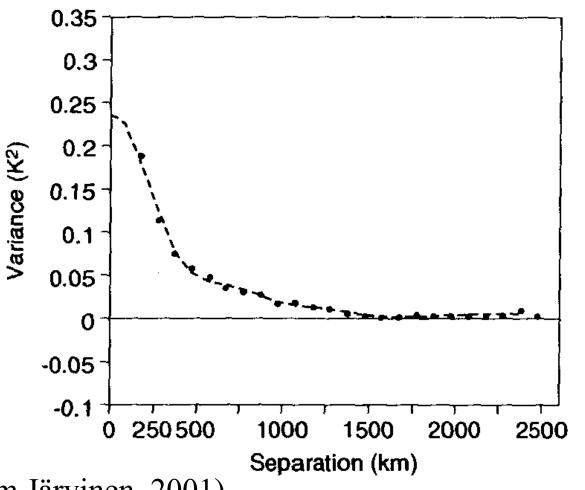
Covariance of d=y-H(x<sub>b</sub>) for AIREP temperatures over USA, binned as a function of observation separation.
