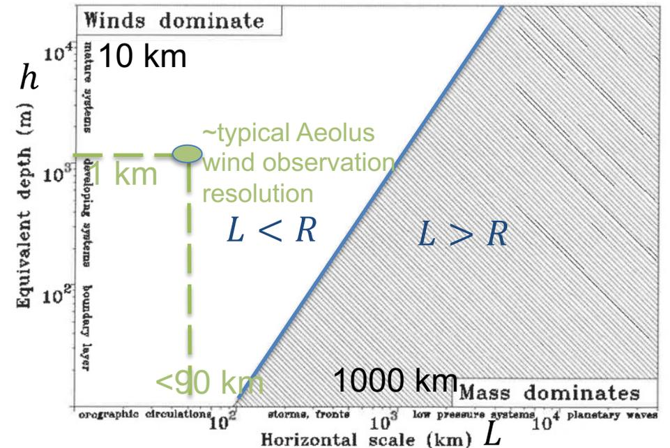
*Figure 2.3. Rossby radius of deformation for a latitude of 45° as a function of horizontal scale and equivalent depth. Open area denotes the range within which the wind field dominates the atmospheric dynamics, and three-dimensional wind measurements are important.*
