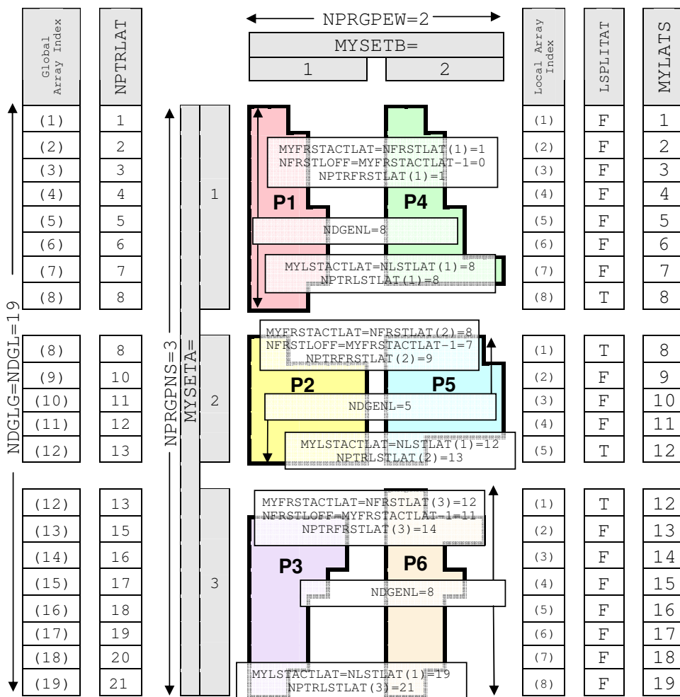
Figure 2.3 Variables describing the Grid Point Decomposition.
